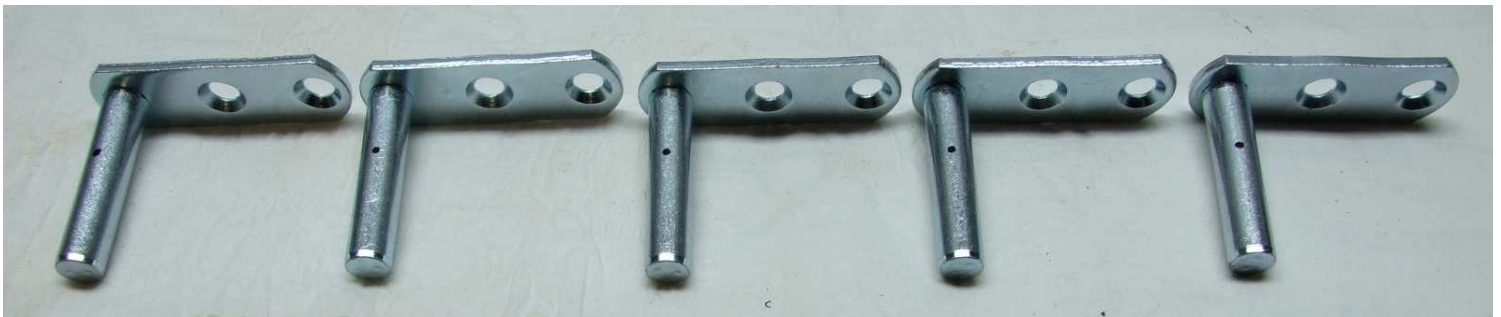
Picture 1. The object(s) before the corrosion test was started. From the left object no. 1-5. The markings indicate where the coating thickness measurements were made.
